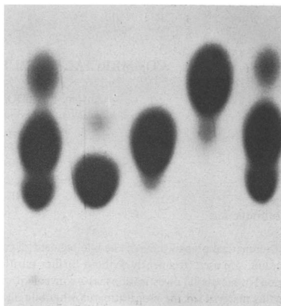
Fig. 2. Thin layer chromatography of bilirubin. L. to r. Pfanstiehl bilirubin, purified bilirubin XIII- \alpha (C), purified bilirubin IX- \alpha (B), purified bilirubin III- \alpha (A), 3X crystallized Pfanstiehl bilirubin.
